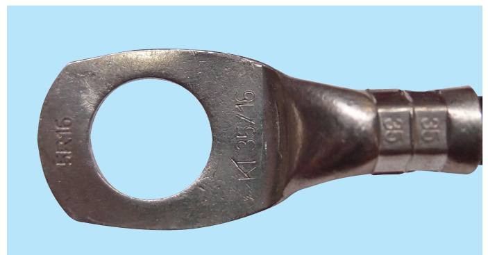
Fig. 2. The cables terminated by a cable lug (cable section 35 mm 2 )
